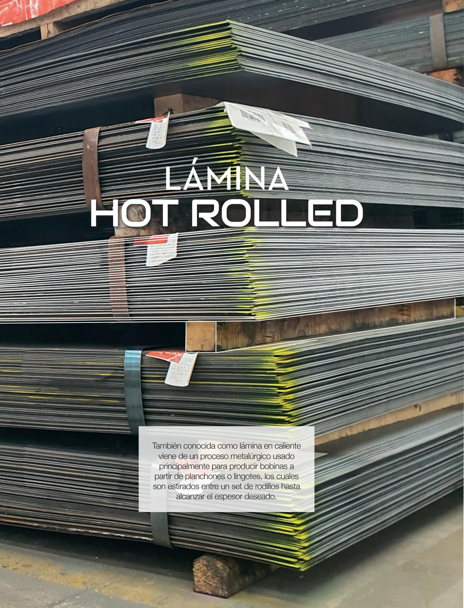
The image shows several large stacks of hot-rolled steel sheets in a warehouse. The sheets are dark grey and have a slightly textured surface. They are stacked on wooden pallets and are secured with metal straps. Some stacks have white labels attached to them. The lighting is bright, highlighting the edges of the sheets.
