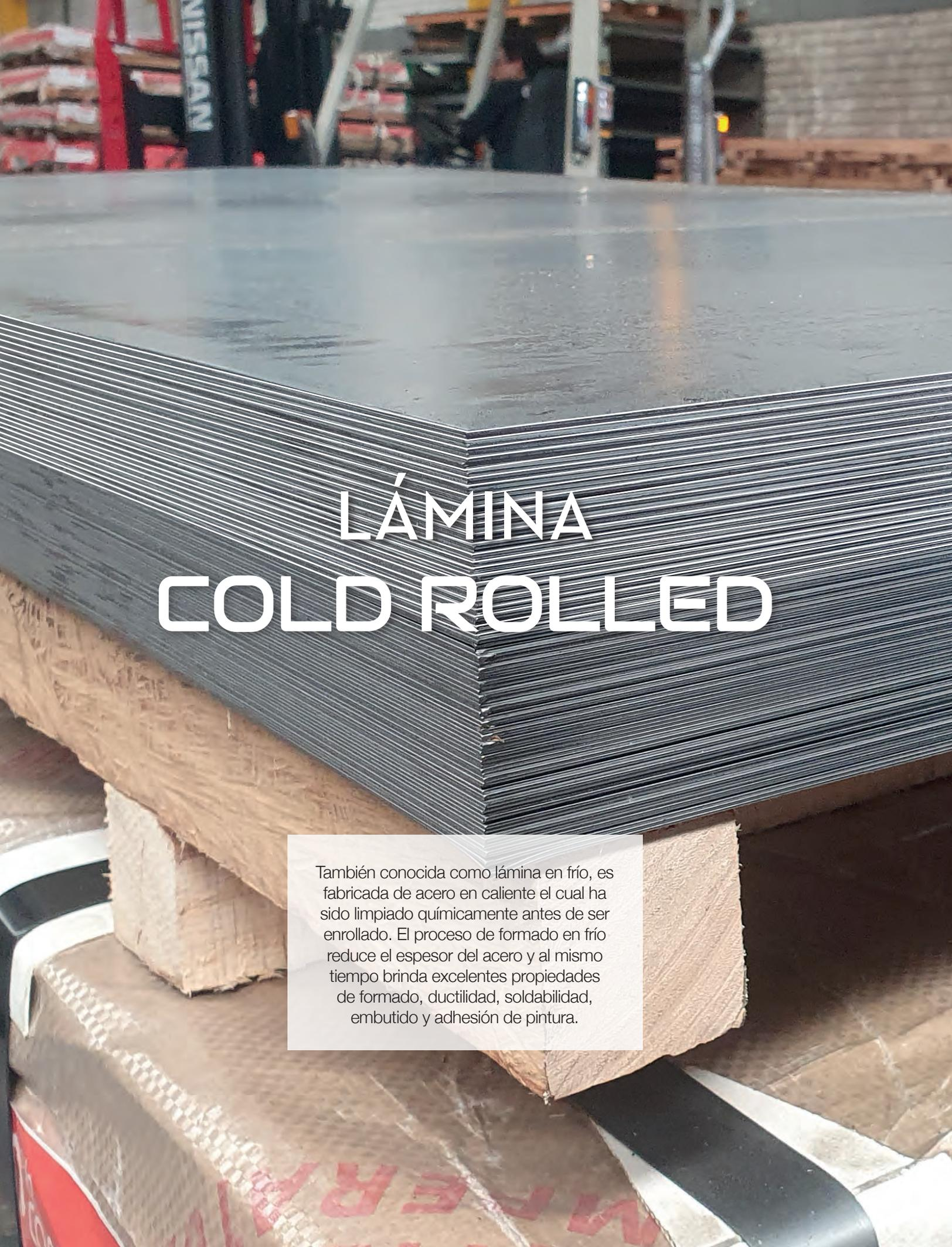
A large stack of cold-rolled steel sheets is shown in a warehouse. The sheets are dark grey and stacked on a wooden pallet. The background shows a forklift and other industrial equipment.
